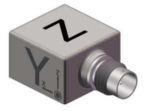
Model 3293A is a low-noise, high sensitivity, miniature LIVM triaxial accelerometer featuring a single, transverse mounted, 4pin electrical connector. This feature allows the 3293A to be used in situations where vertical space is limited. Model 3293A is case grounded. The 3293A is a 500mV/g accelerometer.
